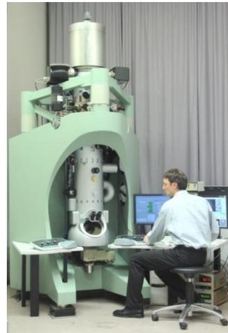
Picture 6: Transmission electron microscope<sup>13</sup>
