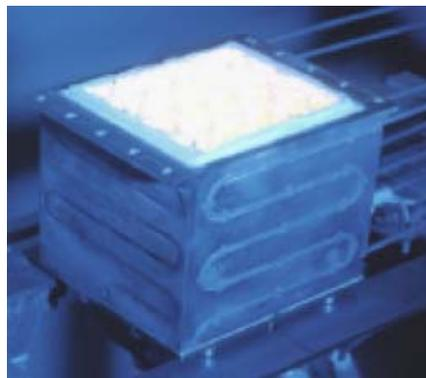
**Picture 3: Cubic Porous Burner in the ZEE03**
