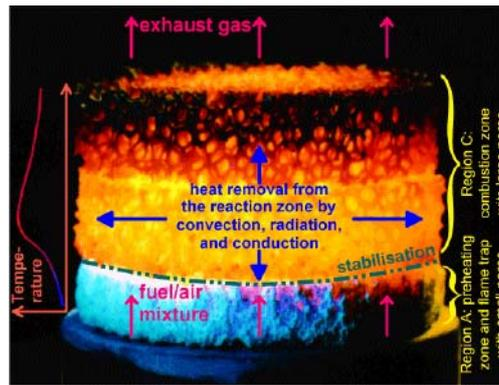
**Picture 2: Porous Burner**
