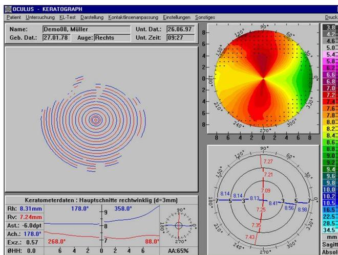
Display of cornea radii by a videokeratoscope
