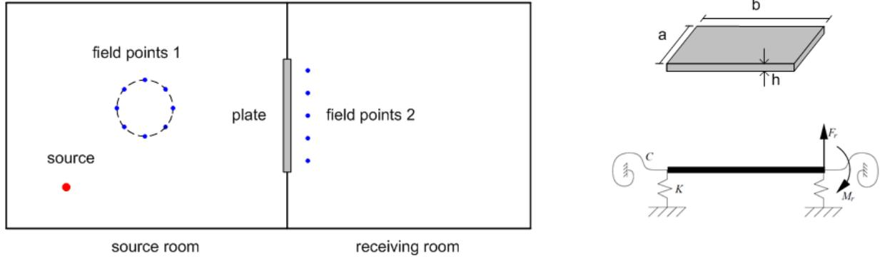
Figure 1 – Illustration of the test facility and the plate with elastic BCs
