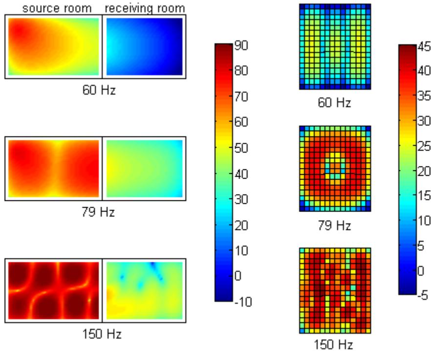
Figure 4 – Sound pressure distribution (left) and normal displacement of the plate (right)
