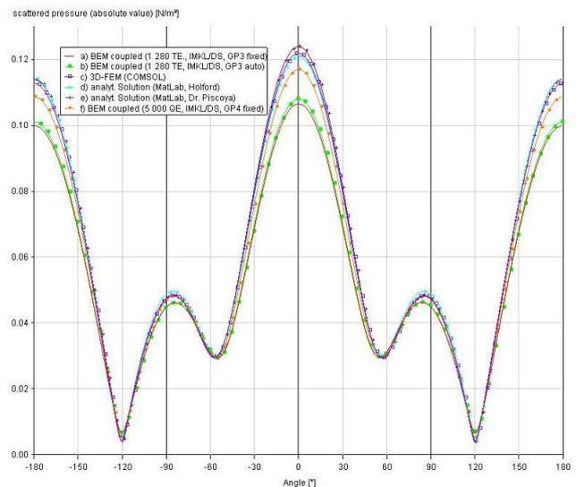
**Figure 7:** 10cm aluminium shell at 1 000 Hz, filled with air and surrounded by water
