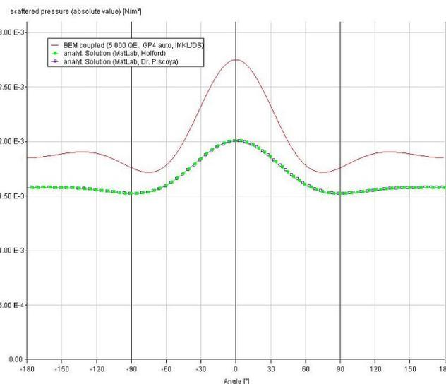
**Figure 13:** 1mm aluminium shell at 1 000 Hz, filled with and surrounded by water
