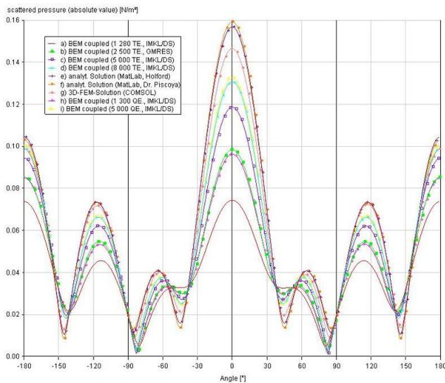
**Figure 5:** 10cm aluminium shell at 1 300 Hz, filled with and surrounded by water
