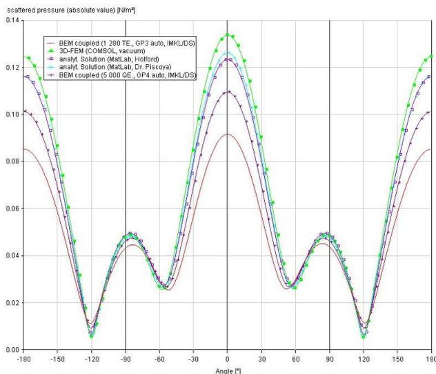
**Figure 9:** 5cm steel shell at 1 000 Hz, filled with air and surrounded by water
