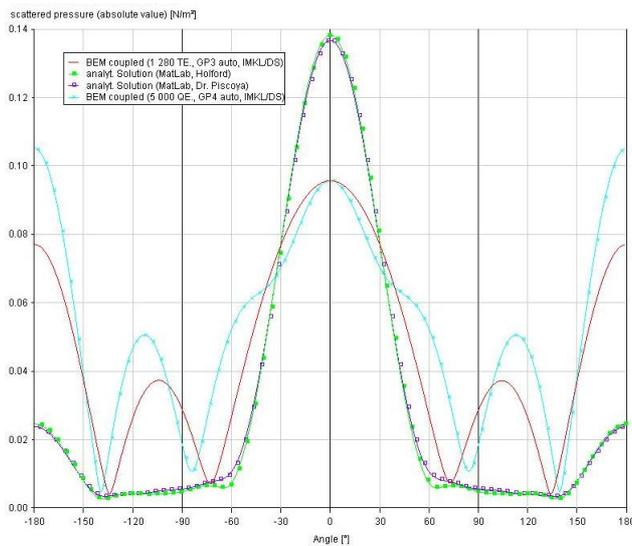
**Figure 12:** 1cm steel shell at 1 000 Hz, filled with air and surrounded by water
