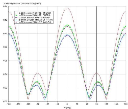
**Figure 6:** 10cm aluminium shell at 1 000 Hz, filled with and surrounded by water
