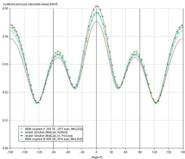
**Figure 8:** 10cm steel shell at 1 000 Hz, filled with air and surrounded by water
