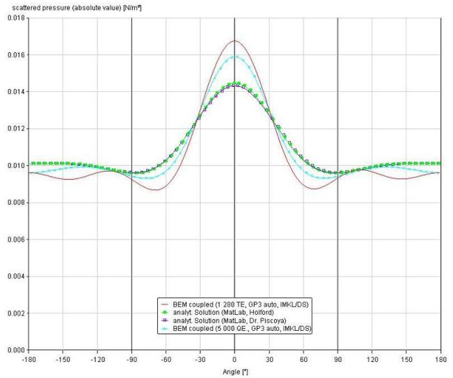
**Figure 10:** 1cm aluminium shell at 1 000 Hz, filled with water and surrounded by water
