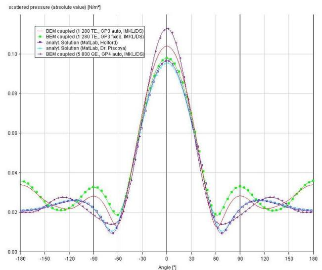
**Figure 11:** 1cm aluminium shell at 1 000 Hz, filled with air and surrounded by water
