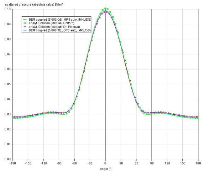
**Figure 14:** 1mm aluminium shell at 1 000 Hz, filled with air and surrounded by water
