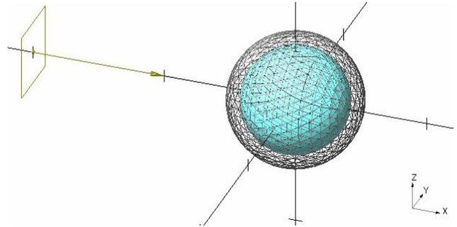
**Figure 3:** Spherical shell with impinging plane wave
