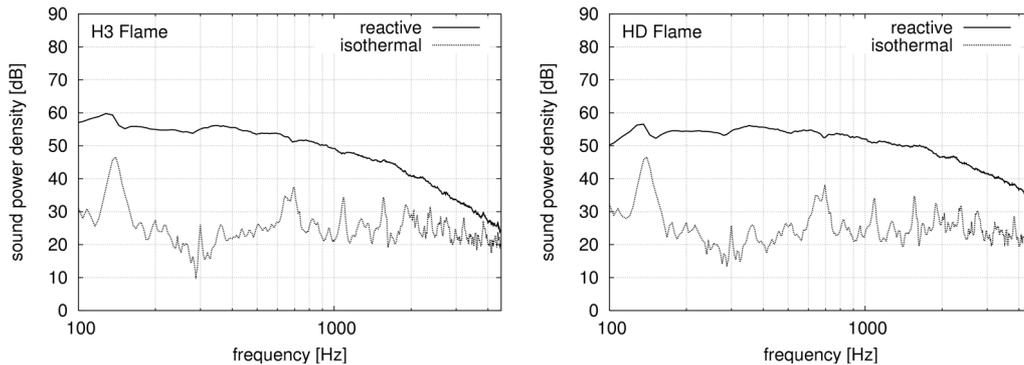
Figure 1: Measurements of the sound power density of the H3 and HD flame as well as the corresponding isothermal cases.
