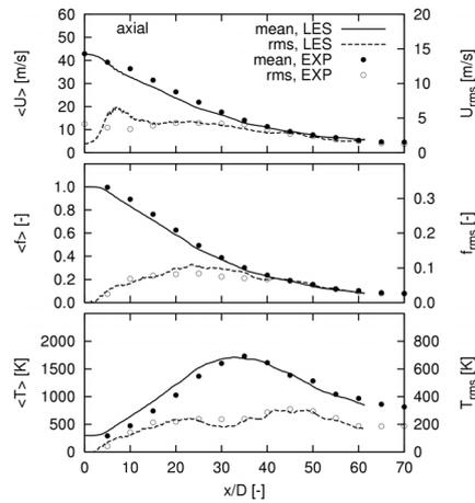
Figure 3: Axial distribution of mean and standard deviation of the axial velocity [m/s], the mixture fraction [-] and the temperature [K] for the H3 flame.
