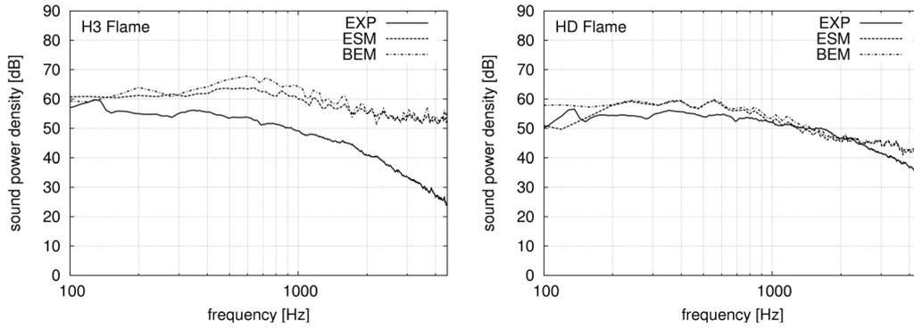
Figure 5: Comparison of the sound power density for the two configurations computed by ESM & BEM to the experimental results.
