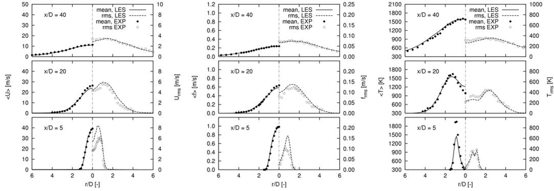
Figure 4: Radial distributions of mean and standard deviation of the axial velocity [m/s], the mixture fraction [-] and the temperature [K] at different axial positions for the H3 flame.
