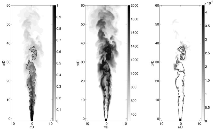
Figure 2: Instationary views of the mixture fraction [-] with the stoichiometric value highlighted by an iso-line, the temperature [K], and the OH mass fraction [-] as a marker for the flame front of the H3 flame.
